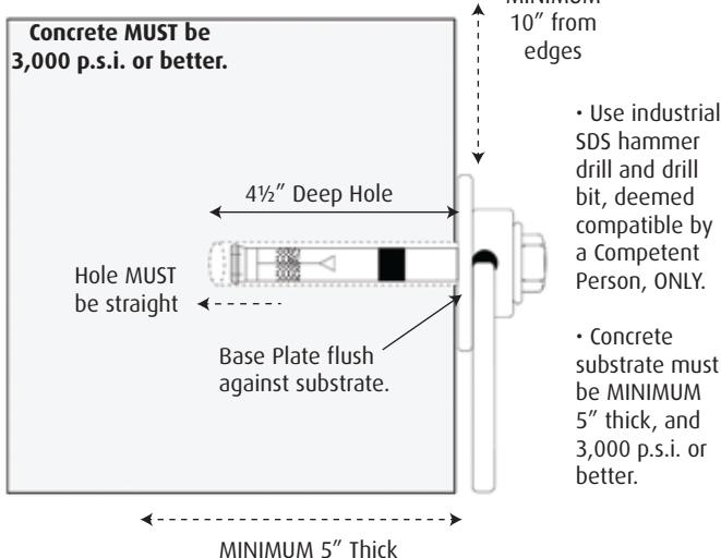
**Not for use in lightweight concrete, brick, grout, or stone.**
